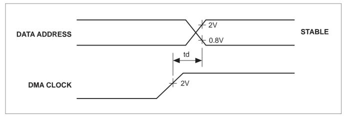
Figure 10: DMA timing
