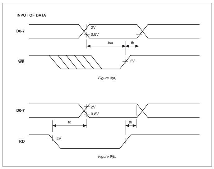
Figure 9: Register timing
