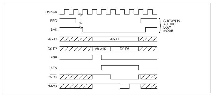
Figure 11: DMA cycle timing
