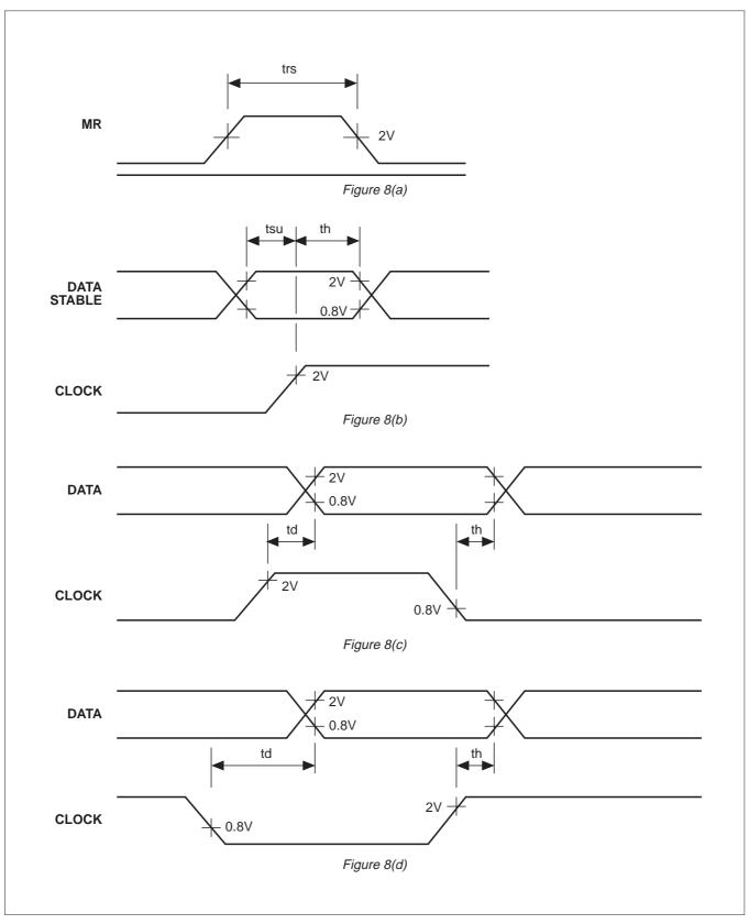
Figure 8: Timing diagram
